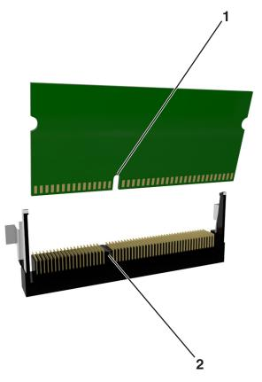
**4** Push the memory card straight into the connector, and then push the card toward the controller board wall until it *clicks* into place.
