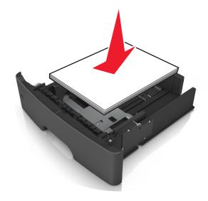
• Make sure the guides in the tray or the multipurpose feeder are properly positioned and are not pressing tightly against the paper or envelopes.
