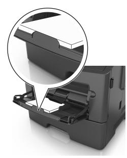
• Load letterhead faceup with the top edge entering the printer first. For two-sided (duplex) printing, load letterhead facedown with the bottom edge entering the printer first.
