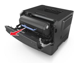
**3** Lift the blue handle, and then pull out the imaging unit from the printer.
